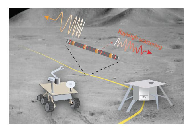
A conceptual lunar fiber seismic network (Background lunar surface image from NASA). The base station provides space and power for the DAS interrogator, data processing unit andtelecommunicating system. The cables (yellow belt) can be deployed by a lunar rover. DAS uses the Rayleigh backscattered light by intrinsic fiber defects (red dots in the enlarged cable section) to detect the longitudinal strain. Credit: Wu et al. (2024), *Seismological Research Letters*
