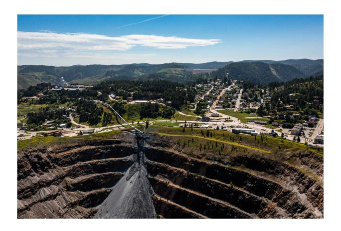
A conveyor carried almost 800,000 tons of rock, excavated a mile underground, into the Open Cut in Lead, South Dakota. Credit: Stephen Kenny, Sanford Underground Research Facility
