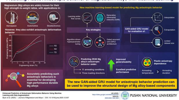
Predicting Plastic Anisotropic Behavior of Magnesium Alloys with Machine Learning
