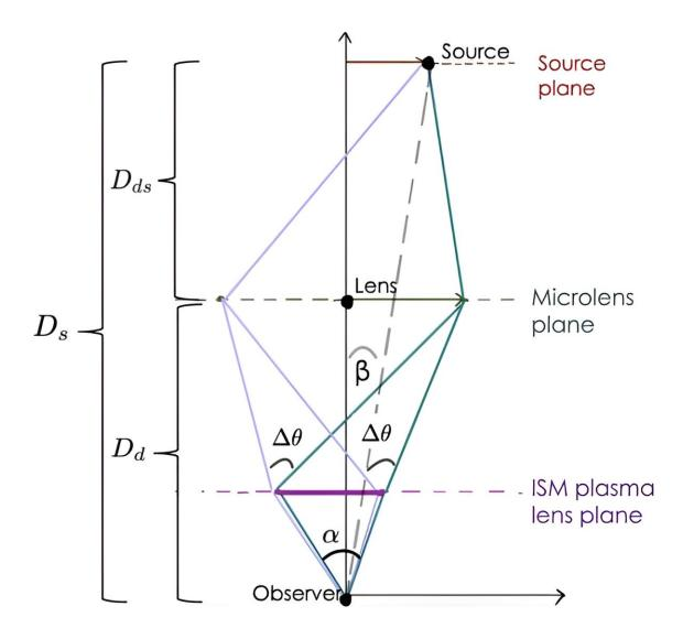
The geometry of an FRB measurement. Credit: Tsai, et al
