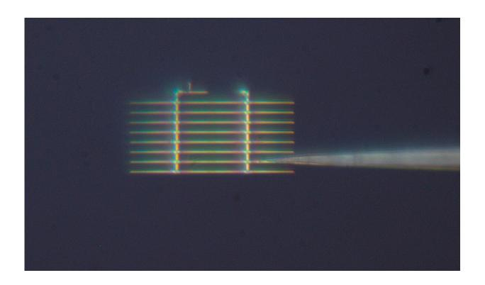
Microscope photograph of a device that could jumpstart work toward the quantum internet. The horizontal lines are diamond waveguides, each about 1,000 times smaller than a human hair. Credit: Atatüre Laboratory, University of Cambridge
