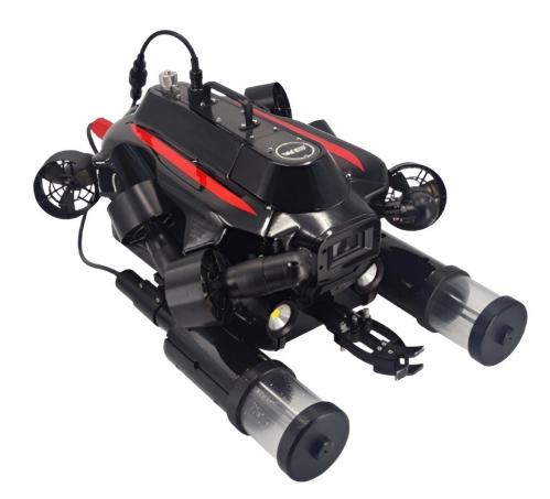
The new and improved underwater drone with two samplers, changeable batteries, and a longer cable, makes collecting seawater samples much easier for researchers. Credit: Okinawa Institute of Science and Technology
