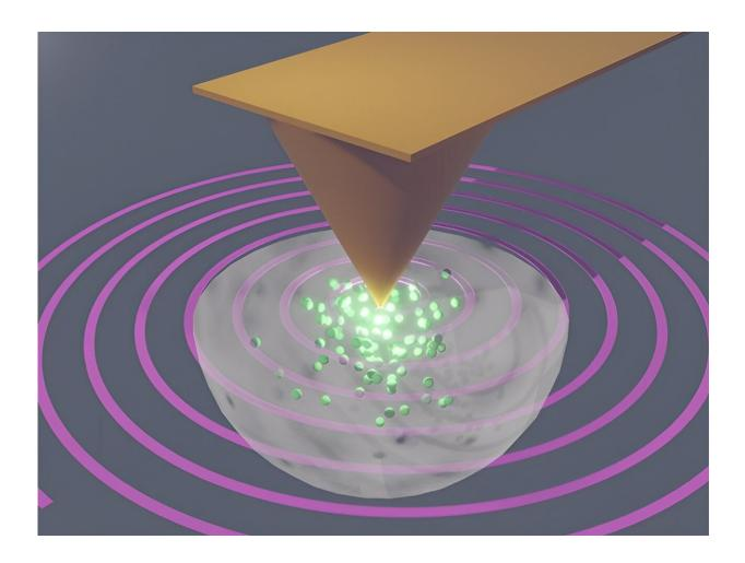
Spiral-tip motion combined with image reconstruction techniques is an approach that can help scientists better understand the behavior of an electric charge at the microscopic level, essential for improving batteries and electronic devices. Credit: Stephen Jesse/ORNL, U.S. Dept. of Energy
