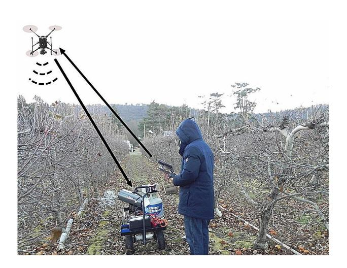
This photo illustration, based on a test researchers conducted of the cyber physical heating system, depicts the concept this study hopefully will lead to, with more research. An orchard worker will remotely pilot an aerial drone that collects temperature readings from apple tree canopies, and it sends locations where heat needs to be applied to protect blossoms to the unmanned ground vehicle. The vehicle then will head to those spots and heat them, supporting
