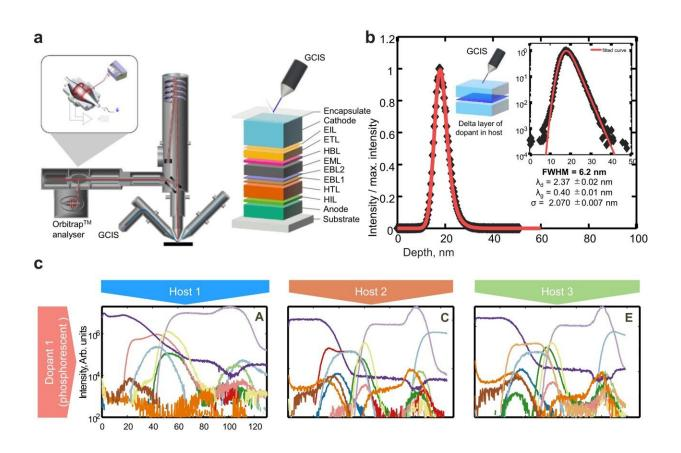
High-resolution chemical depth profiling of blue OLED devices of varying architecture. Credit: *Nature Communications* (2023). DOI: 10.1038/s41467-023-43840-9
