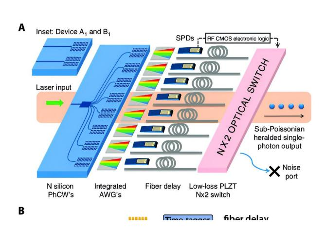
Experimental setup for heralded photon using (A) spatial multiplexing technique [18] and (B) temporal multiplexing technique [20]. Credits: Benjamin J. Eggleton (A) and Yunhong Ding (B). *Advanced Devices & Instrumentation* (2023). DOI: 10.34133/adi.0032
