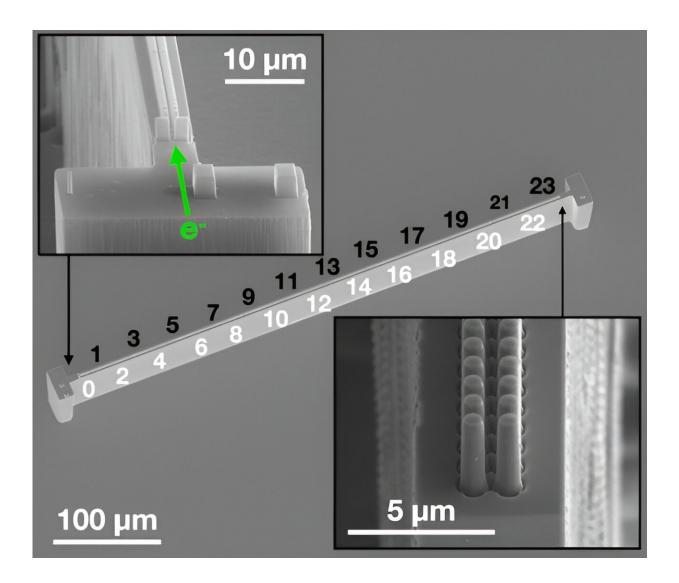
Scanning electron micrograph of a half-millimeter long dielectric laser accelerator through which electrons travel and accelerate. Cells labeled as black are longitudinally focusing and transversely defocusing (LFTD), while white are
