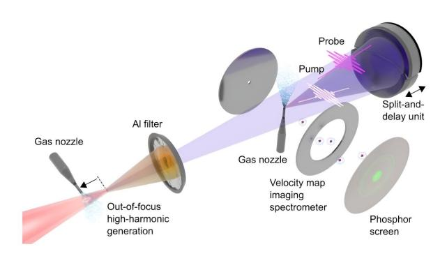
Experimental setup for attosecond-pump attosecond-probe spectroscopy. NIR pulses are focused behind a pulsed gas jet, where attosecond pulses are generated. At some distance from the gas jet, spherical half-mirrors are used to spectrally select and focus the attosecond pump and the probe pulses. The generated ions are recorded using a velocity-map imaging spectrometer. Credit: MBI / Mikhail Volkov
