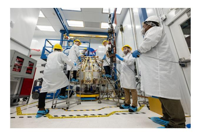
A team of engineers prepares to integrate TRIDENT—short for The Regolith Ice Drill for Exploring New Terrain—into the belly of NASA's first robotic moon rover, VIPER—short for the Volatiles Investigating Polar Exploration Rover. Credit: NASA/Bill Stafford
