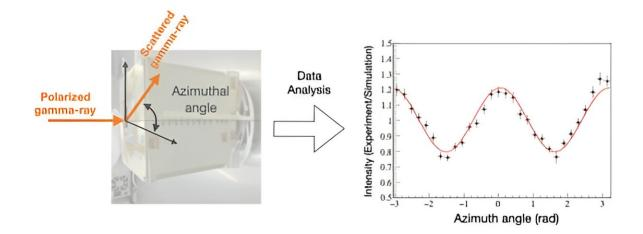
Scattering angle distribution (right) of polarized gamma rays as captured by the multi-layer Compton camera (left). The black dots show the distribution and red line shows the modulation curve. Credit: RIKEN
