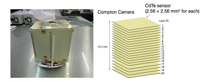
The CdTe Compton Camera (left) and the 20 layers inside (right). Credit: RIKEN
