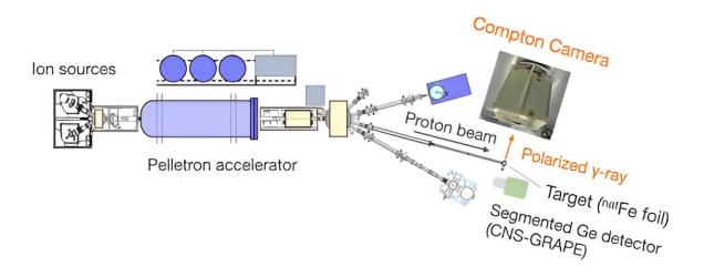
The RIKEN tandem (Pelletron) accelerator and beam lines. Credit: RIKEN
