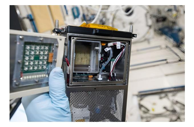
This image shows the Plant Experiment Unit (PEU) hardware for the Plant UV-B investigation. Credit: NASA
