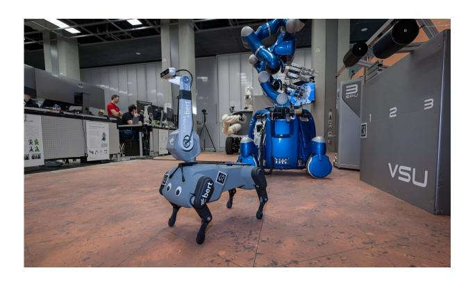
DLR's four-legged robot Bert explores and monitors the unfamiliar environment. The Surface Avatar Experiment rehearsed an important scenario for future exploration missions on the moon and Mars. Bert is being developed at the DLR Institute of Robotics and Mechatronics and can walk, trot, gallop, perform a passing gait and even climb. This enables him to cover long distances and at the same time move around in rough terrain or small caves. Credit: DLR
