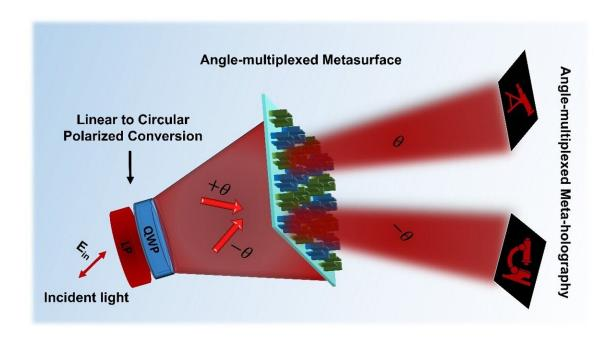
Versatile meta-holographic display featuring different images based on viewing angle. Credit: POSTECH
