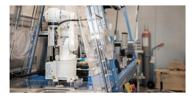
This robotic arm transfers glass vials into a centrifuge. It is part of a robot unit that produces catalysts completely autonomously according to the specifications of an AI model. Credit: ETH Zurich / Michel Büchel
