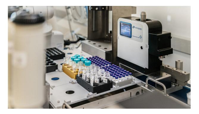
Precision scale of the robotic system. The system transfers solid and liquid raw chemicals into the glass vials in which the synthesis takes place. Credit: ETH Zurich / Michel Büchel
