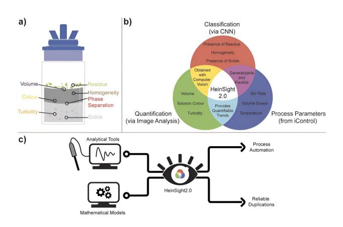
(a) Universal vision-based outputs in workups monitored by HeinSight2.0; (b) overview of interrelated components of HeinSight2.0: Classification outputs (from CNN), quantification outputs (from image analysis), and process variables from iControl; (c) integrations and applications of HeinSight2.0 CV system. Credit: *Chemical Science* (2023). DOI: 10.1039/D3SC05491H
