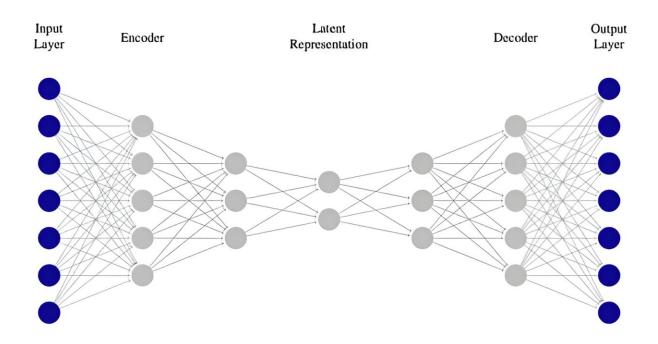
This simple schematic illustrates the general architecture of an autoencoder. It takes input, encodes it into a latent representation of the input, then decodes it and outputs it. Credit: Rogers et al. 2024
