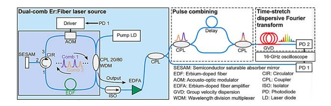
Setup of the dual-comb fiber laser oscillator, external pulse combination, and real-time detection. Credit: *Science Advances* (2024). DOI: 10.1126/sciadv.adk2290
