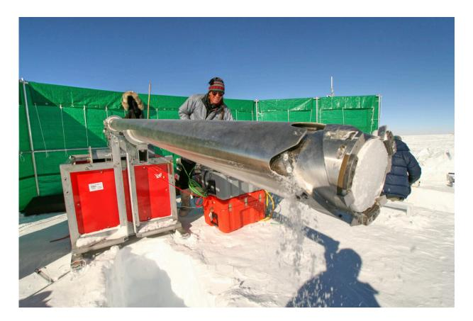
A U.S. ice core driller collecting a core used in this study as part of the Norwegian-U.S. scientific traverse of East Antarctica. Credit: Stein Tronstad
