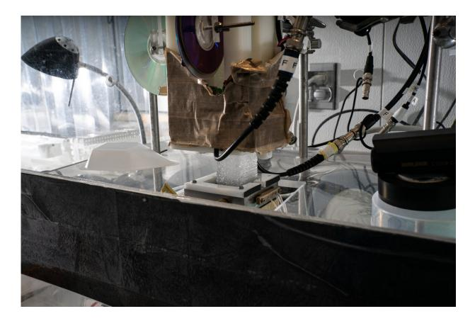
The ice core sample being processed on the unique ice core analytical system at DRI's Ice Core Lab. Credit: Jessi LeMay/DRI
