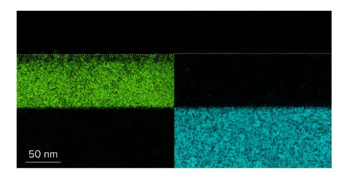
A transmission electron micrograph of the material on its substrate. It shows the distribution of iron atoms in the iron selenide thin film (left) and lanthanum atoms in the substrate (right). Credit: *Physical Review B* (2023). DOI: 10.1103/PhysRevB.108.L100501
