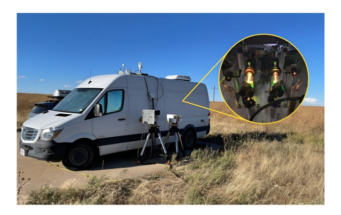
A research van housed a mid-infrared laser system (inset) and telescope, which directed light across the open air to a mirror several hundred meters away. Credit: K. Cossel/NIST
