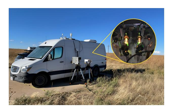
A research van housed a mid-infrared laser system (inset) and telescope, which directed light across the open air to a mirror several hundred meters away.
