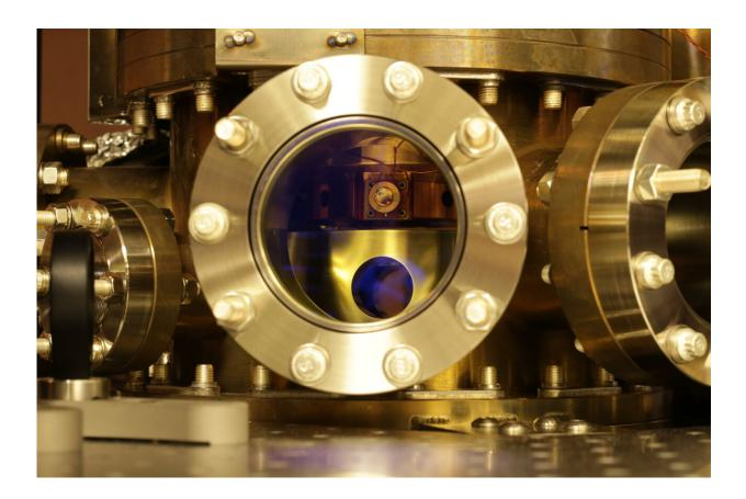
A photo of the atomic clock setup complete with the bisecting cavity. Credit: JILA/Ye Group
