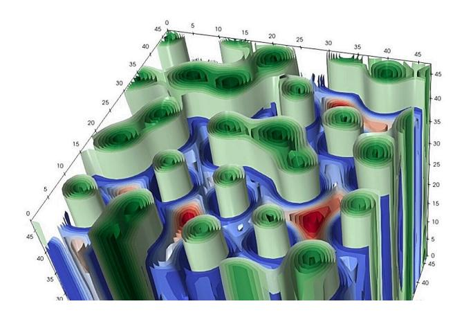
A typical 3D configuration in the superconducting vortex phase in the (hyper)magnetic field background of about 150 exatesla. The equipotential surfaces of the superconducting W condensate are shown in blue and red, and the ones of the Higgs condensate are shown in green. These quantities are shown in complementary regions. Credit: Vladimir Goy, from *Physical Review Letters* (2023). DOI: 10.1103/PhysRevLett.130.111802
