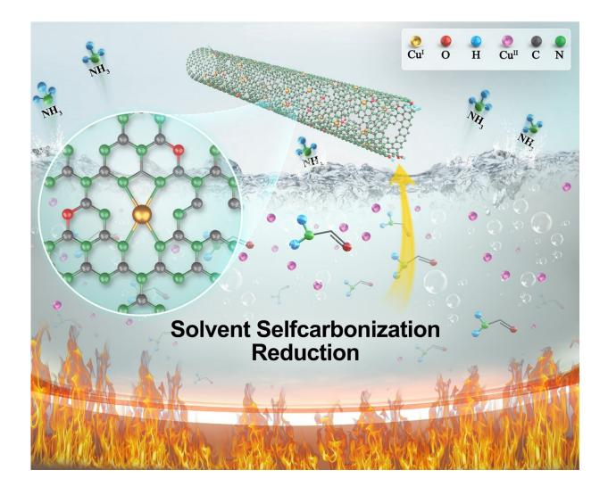
Schematic illustration showing the preparation process of Cu<sup>I</sup> SAEs. Credit: Liu Hongji
