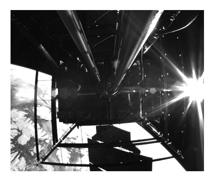
The DOLCE structure completely deployed, over the Canadian Arctic, on September 29, 2023. DOLCE structure's TRAC longerons and battens are clearly visible above the Arctic ice. The fiberglass batten connectors are shining under the Sun (right part). Credit: Space Solar Power Project/Caltech
