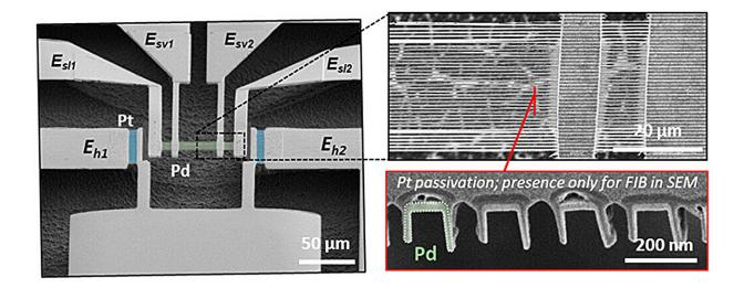
Electron microscopy of the coplanar heater-integrated hydrogen sensor. (Left) photo of the entire device. (Top right) Pd nanowire suspended in the air. (Bottom right) Cross section of Pd nanowire. Credit: *ACS Nano* (2023). DOI: 10.1021/acsnano.3c06806
