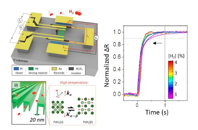
(Left) The conceptual drawing of the structure of the coplanar heater-integrated hydrogen sensor. Pd nanowire is stably suspended in the air even with its thickness of 20 nm. (Right) A graph of hydrogen sensor performance operating within 0.6 seconds for hydrogen at a concentration of 0.1 to 4%. Credit: *ACS Nano* (2023). DOI: 10.1021/acsnano.3c06806
