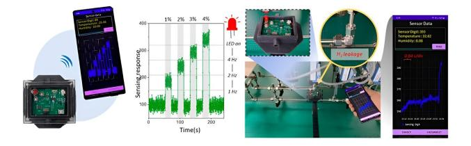
(Left) Real-time hydrogen detection results from the coplanar heater-integrated hydrogen sensor integrated and packaged in wireless communication and an app for mobile phone. (Middle) LED blinking cycle control in accordance with the hydrogen concentration level. (Right) Results of performance confirmation of the detection within 1 second in a real-time hydrogen leak demo. Credit: *ACS Nano* (2023). DOI: 10.1021/acsnano.3c06806
