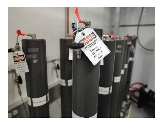
Pressure cores of methane hydrate. Scientists collected the cores during a 2023 mission led by The University of Texas at Austin. The cores are now kept in a special lab at the UT Austin Jackson School of Geosciences. Credit: UT Austin / Jackson School of Geosciences
