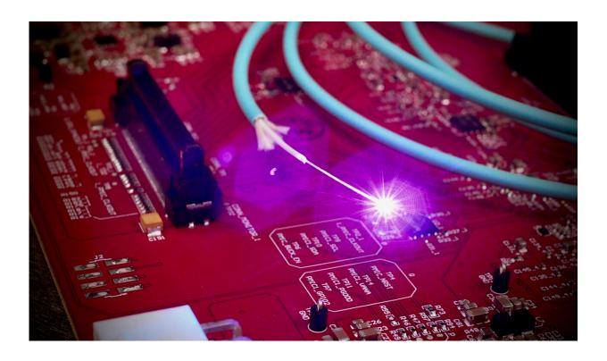
Light traveling through an optical fiber sitting on top of a conventional electronic circuit board. Credit: Heriot-Watt University
