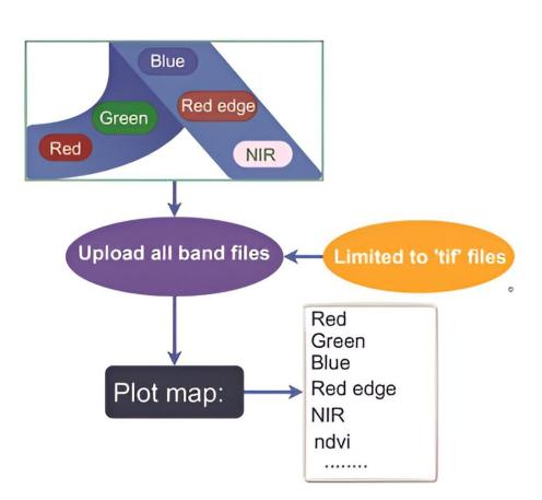
The workflow for the VIs generation process that is implemented in VIs generation. Credit: *Plant Phenomics*
