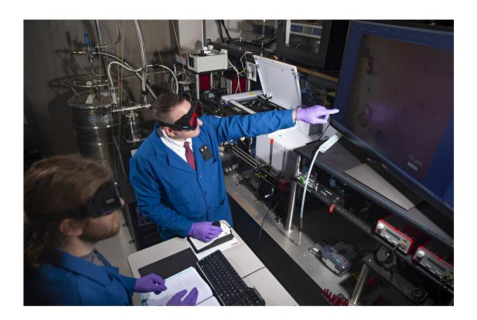
In his laboratory at the Center for Integrated Nanotechnologies in Los Alamos, Michael Pettes and graduate research assistant Micah Vallin examine the vibrational signatures of a two-dimensional magnetic material under cryogenic conditions using a customized confocal Raman spectroscopy microscope. Credit: Los Alamos National Laboratory
