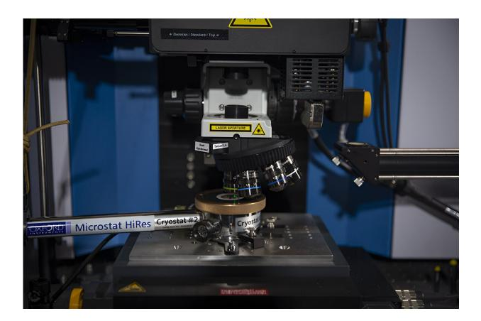
A close-up view of confocal Raman spectroscopy, in which a 532-nanometer laser (seen in green) is being used to probe the vibrational structure of van der Waals materials contained in a high vacuum cryostat at 3.8 Kelvin. Credit: Los Alamos National Laboratory
