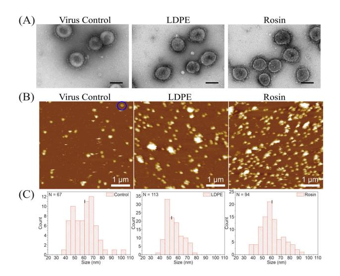
Studying the impact of rosin-functionalized plastic and standard LDPE on the structure of HCoV-OC43 using (A) TEM and (B) AFM in liquid. The scale bar corresponds to 100 nm and 1  $\mu$ m in the TEM and AFM images, respectively. In panel B, the blue circle highlights a doughnut-shaped virus. (C) The histogram
