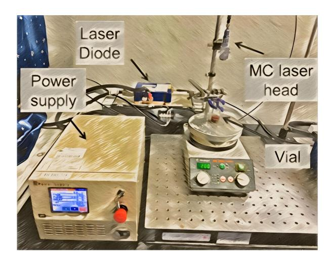
One of the setting examples for PLAL experiment in the organic synthetic lab. By using MCL, just less than half of the usual lab table space is needed. Credit: Yumi Yakiyama and Hidehiro Sakurai, Osaka University, Japan.
