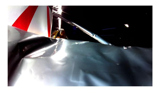
This handout image released by Astrobotic shows the Peregine Lunar Lander's damaged Multi-Layer Insulation (MLI) following an anomaly.
