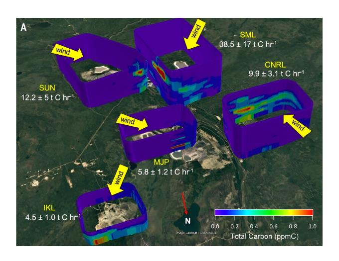
Examples of box flights around five major surface mining facilities on different days show elevated downwind total gaseous organic carbon with total emissions derived with TERRA (supplementary materials, materials and methods). Numeric values in white indicate average TC emission rates. Credit: *Science*
