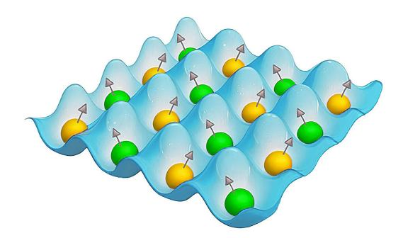
Magnetic structure of a material. The colored spheres represent atoms and the arrows stand for their magnetic moments. The curved surface illustrates how the atoms assume the most energetically favorable positions. The magnetic moments, likewise, adopt the most energetically favorable orientations. Credit: Pavel Odinev/Skoltech PR
