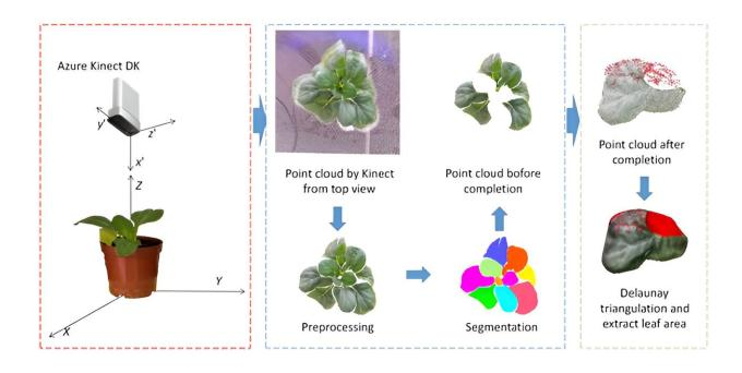
The workflow of the completion of plant point cloud. Credit: Plant Phenomics
