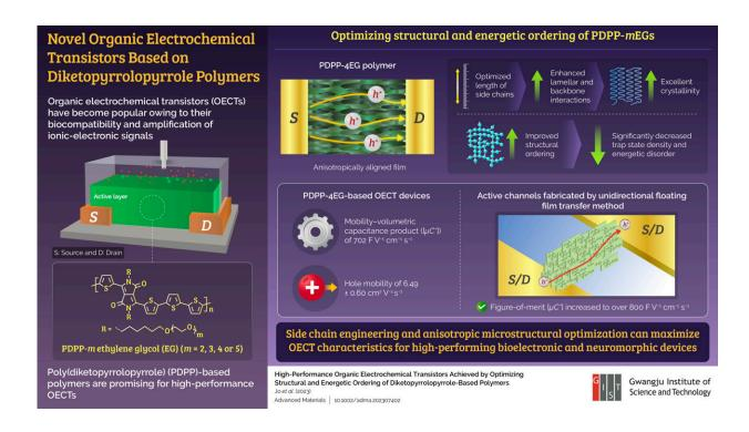
Molecular design and structural alignment to optimize the performance of OECTs produces a product of charge carrier mobility and volumetric capacitance equal to 702 F V<sup>-1</sup> cm<sup>-1</sup> s<sup>-1</sup> through spin casting and 804 F V<sup>-1</sup> cm<sup>-1</sup> s<sup>-1</sup> when fabricated using unidirectional floating film transfer method. Credit: Myung-Han Yoon from GIST
