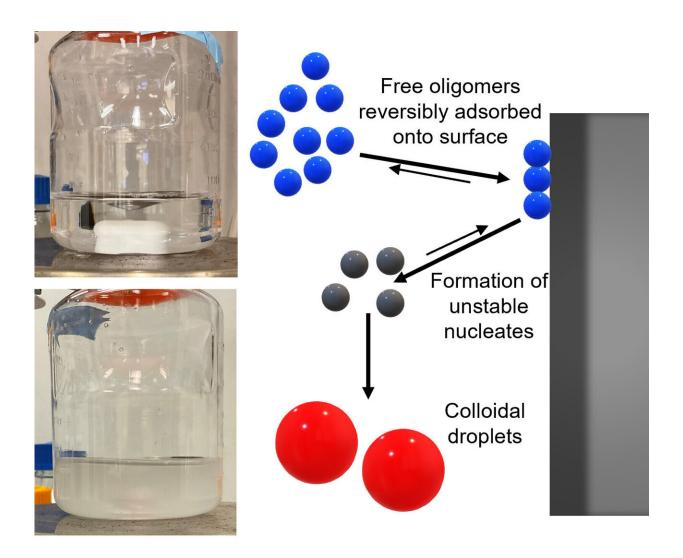
Schematic of the proposed mechanism for the surface-mediated spontaneous emulsification process (ouzo) effect. Photos of the SMG stirring experiment are
