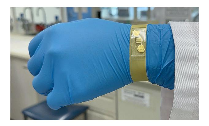
The team used a low-cost and scalable technique to deposit super thin tin dioxide onto a base material--even on a flexible material, which other approaches had challenges achieving. Credit: Seamus Daniel, RMIT
