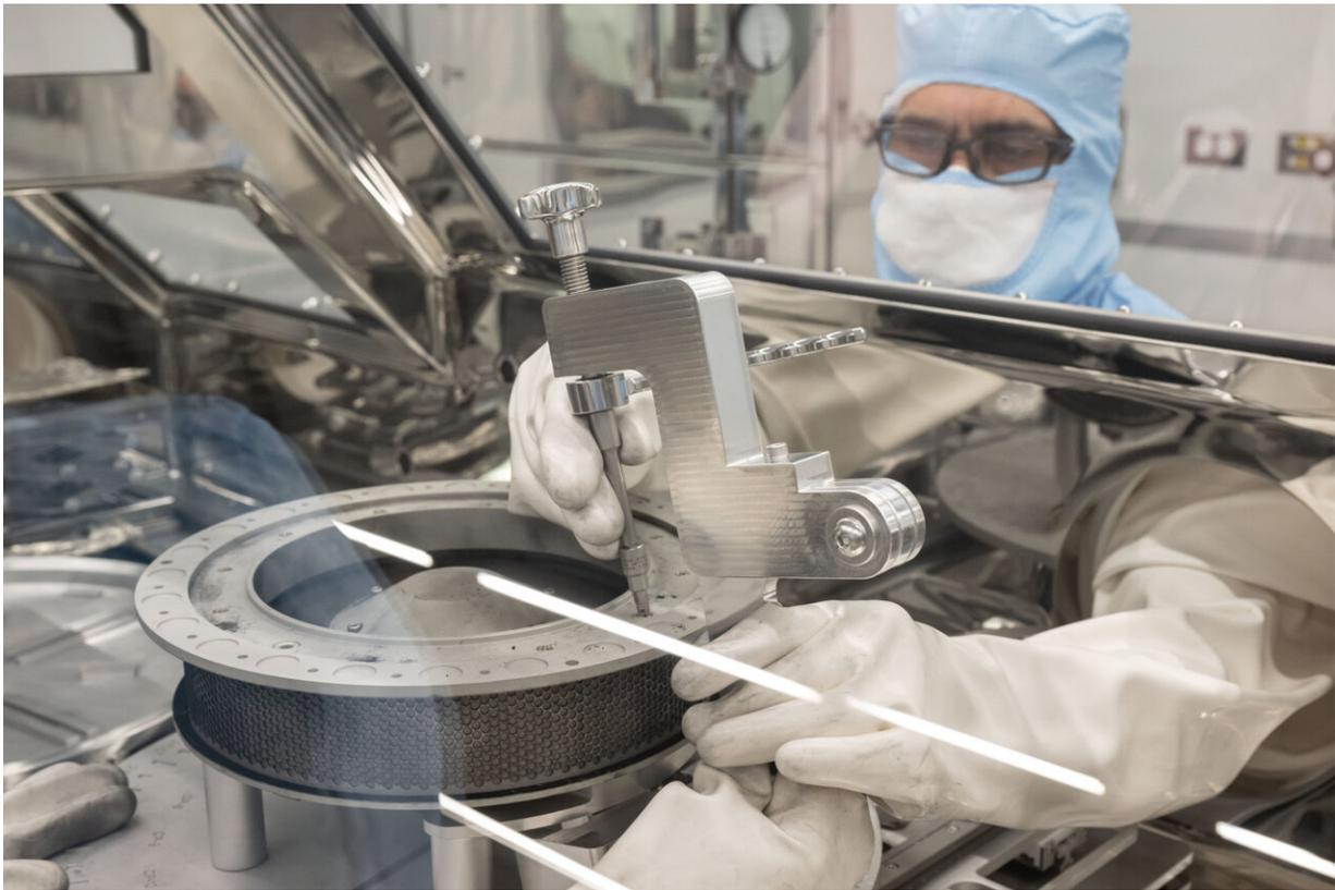
NASA's OSIRIS-REx curation engineer, Neftali Hernandez, attaches one of the tools developed to help remove two final fasteners that prohibited complete disassembly of the TAGSAM (Touch-and-Go Sample Acquisition Mechanism) head that holds the remainder of material collected from asteroid Bennu. Engineers on the team, based at NASA's Johnson Space Center in Houston, developed new tools that freed the fasteners on Jan. 10. Credit: NASA/Robert Markowitz
