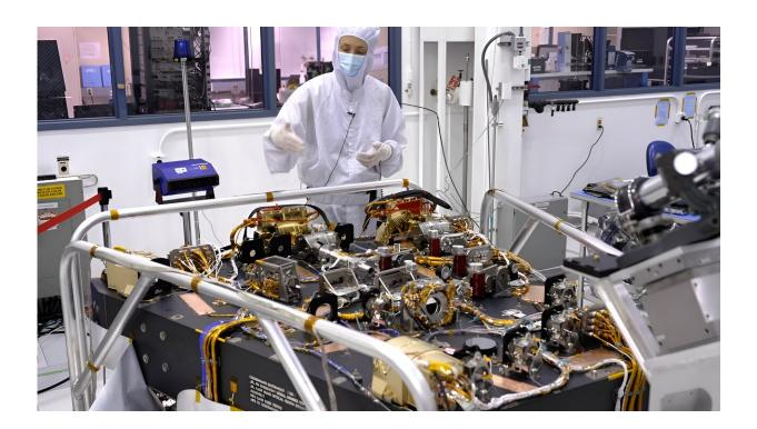
JPL scientist Vanessa Bailey stands behind the Nancy Grace Roman Coronagraph, which has been undergoing testing at JPL. About the size of a baby grand piano, the Coronagraph is designed to block starlight and allow scientists to see the faint light from planets outside our solar system. Credit: NASA/JPL-Caltech
