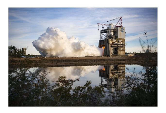
NASA completed a full-duration, 500-second hot fire of an RS-25 certification engine Jan. 17, continuing a critical test series to support future SLS (Space Launch System) missions to the moon and beyond as NASA explores the secrets of the universe for the benefit of all. Credit: NASA/Danny Nowlin
