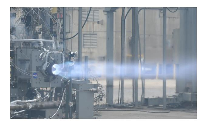
Engineers at NASA's Marshall Space Flight Center in Huntsville, Alabama, conduct a successful, 251-second hot fire test of a full-scale Rotating Detonation Rocket Engine combustor in fall 2023, achieving more than 5,800 pounds of thrust. Credit: NASA
