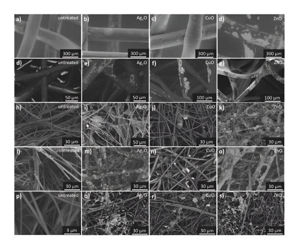
Secondary electron scanning electron micrographs of untreated and modified air filter media, spray-coated with Ag2O, CuO and ZnO particles. Credit: IMDEA Materials Institute
