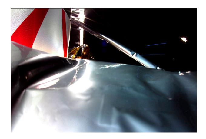
In this image released by Astrobotic Technology, an image from a mounted camera shows a disturbed section of insulation on the Peregrine lander, while on its way to land on the moon, Monday, Jan. 8, 2024. Astrobotic said the moon landing is in jeopardy because of a fuel leak that developed hours after the spacecraft's launch. Credit: Astrobotic Technology via AP
