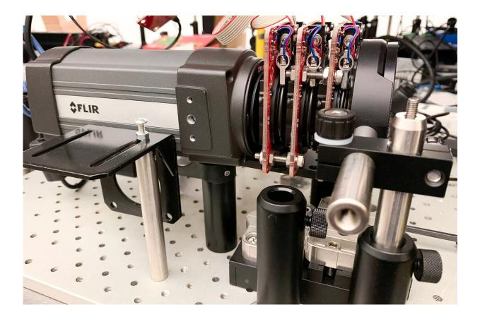
The stack of spinning metasurfaces breaks down thermal light into its spectral and polarimetric components. The researchers combined the metasurface stack with a traditional long-wave infrared camera and computational imaging algorithms to create a compact and robust spectral thermal imaging system. Credit: Xueji Wang, Purdue University
