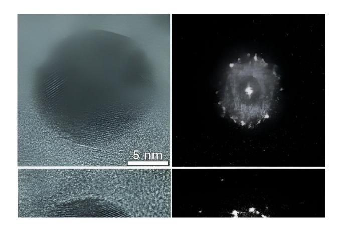
High resolution transmission electron microscope images of Au nanoparticles before (above) and after (below) encapsulation. Credit: Northwestern University
